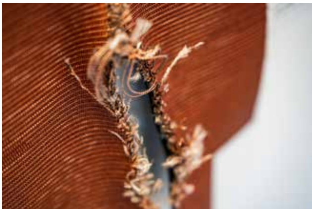
Unique weave designs using high quality, super-strength individual fibres and yarns stops rips and tears in their tracks. (Image courtesy of Fenner Dunlop).
