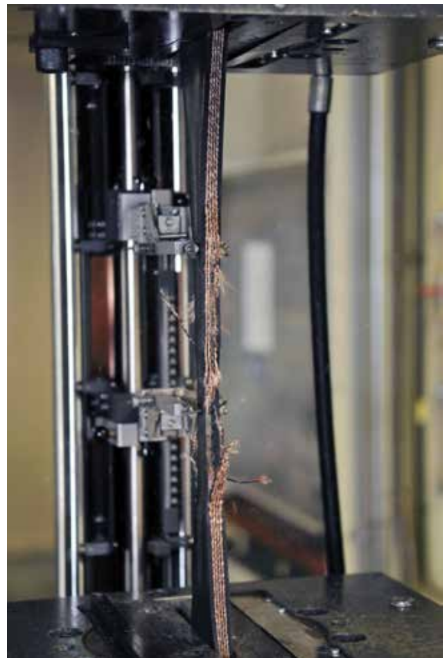
Elongation at break is the amount of elongation at the moment the belt breaks.
