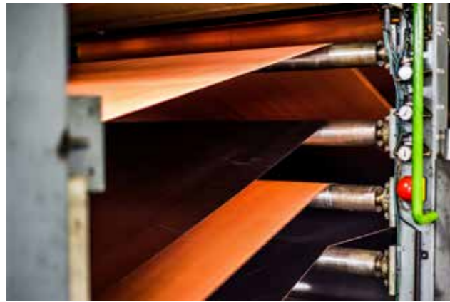
The fabric inner plies and thin layers of rubber (skim) are compressed together to create the belt carcass.
