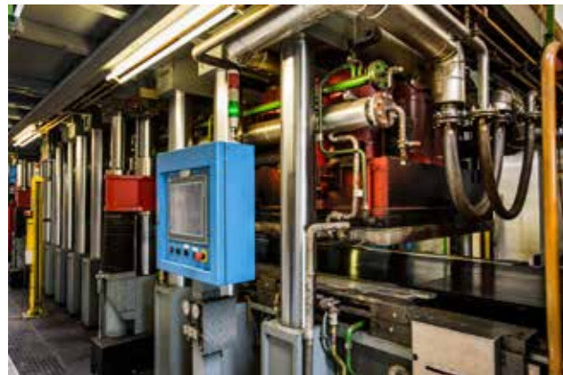
Temperatures and pressure levels of the vulcanizing press need to be accurate and uniform.
