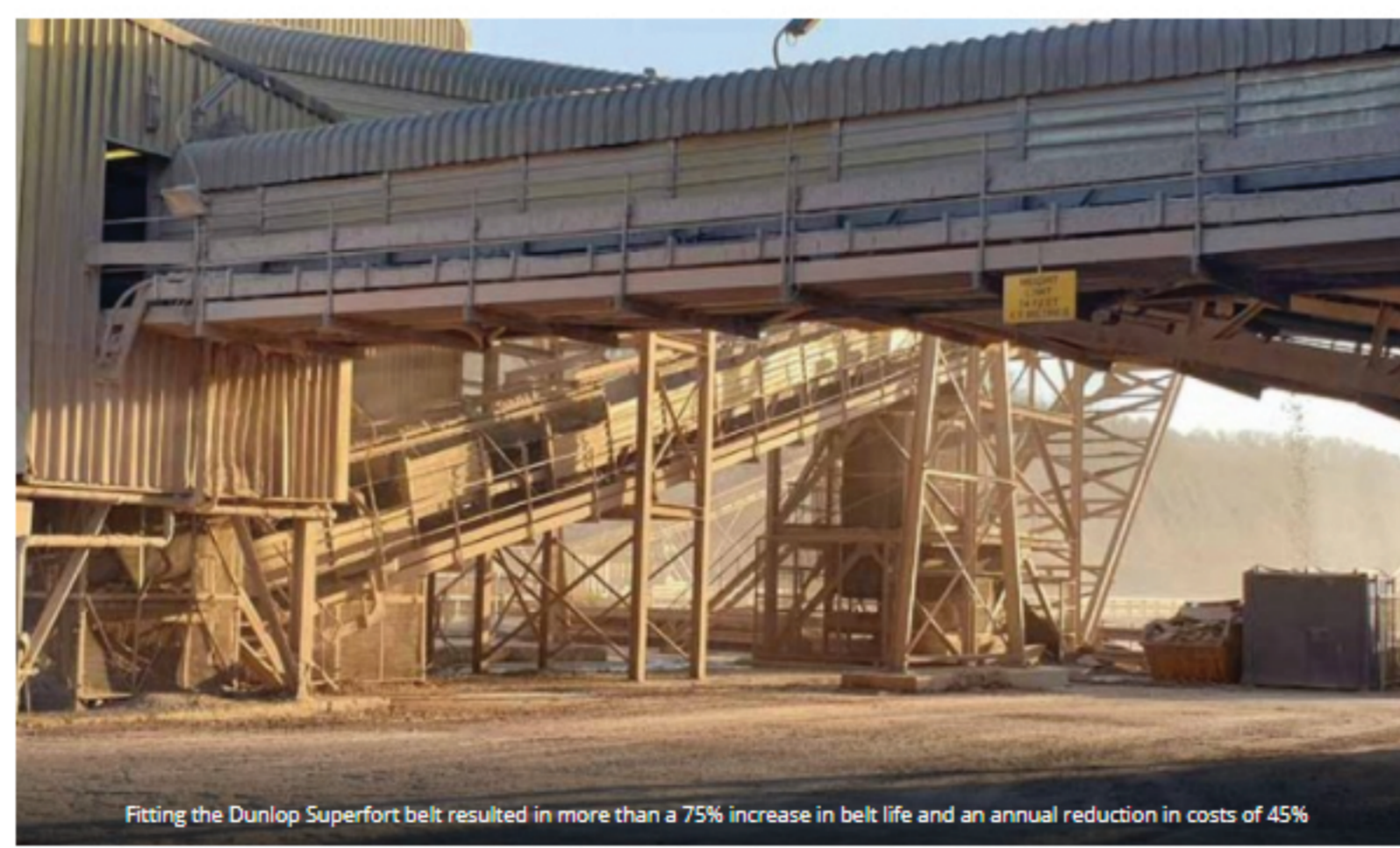
Fitting the Dunlop Superfort belt resulted in more than a 75% increase in belt life and an annual reduction in costs of 45%
