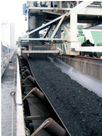
Running straight and true - polyester and nylon fabric (EP) in multi-ply belts usually has the best balance of mechanical properties.
