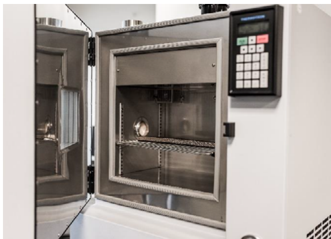
Rubber samples are frozen using liquid nitrogen
