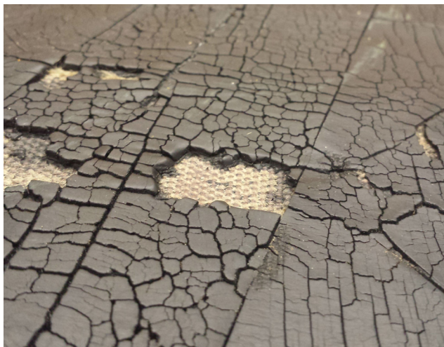
Figure 4. Heat is the ultimate belt killer.
