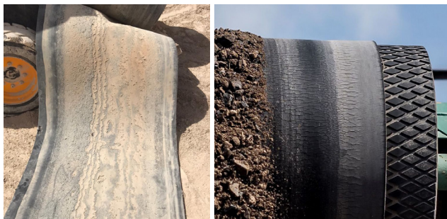
Figures 1 & 2. Insufficient resistance to abrasion is a prime cause of premature belt replacement (left) and the seriously damaging effects of ozone and ultraviolet light (right).
