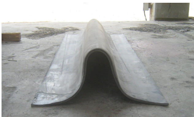
Figure 3. Serious distortion – the effect of oil on a flat rubber belt.
