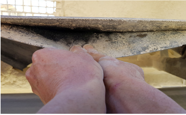
Figure 5. Delamination – if the inner carcass becomes too hot, the belt will literally fall apart.
