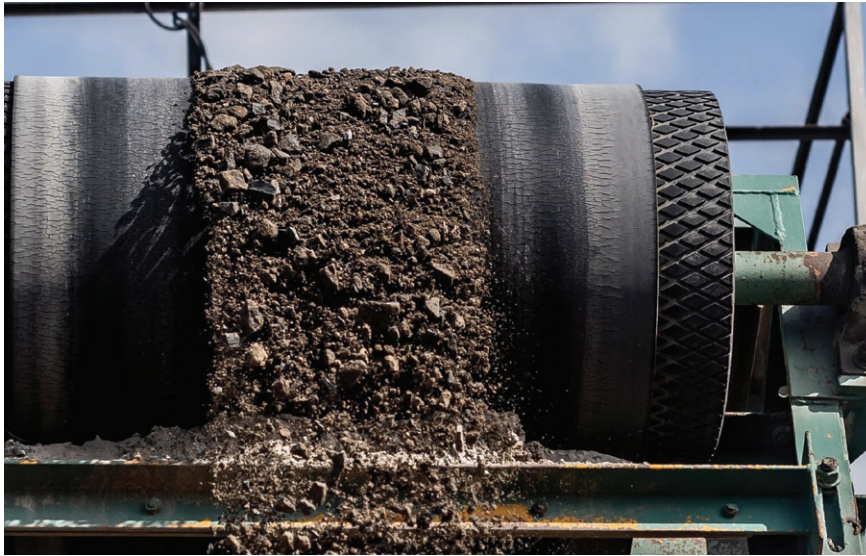
Left: Pollution problems – fine particles of dust penetrate cracks and are then discharged (shaken out) on the return (underside) run of the belt. Right: Close up of the cracks
