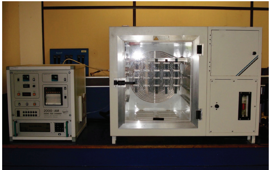
Samples are checked for cracking at two-hourly intervals
