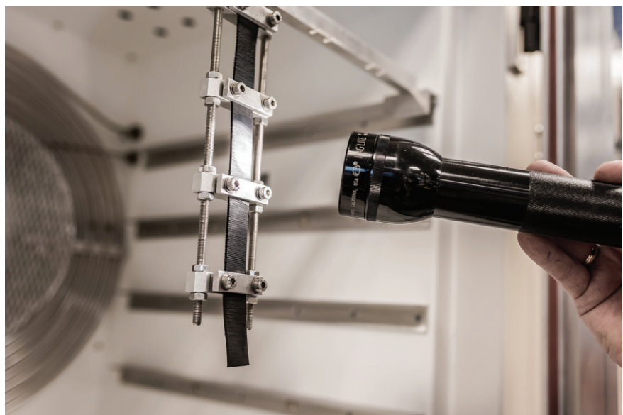
Samples are checked for cracking at two-hourly intervals
