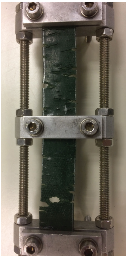
Some rubber literally disintegrates within hours
