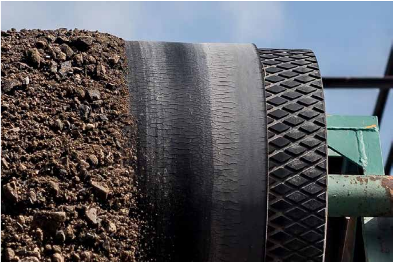
The first signs - small cracks appear in the surface of the rubber.
