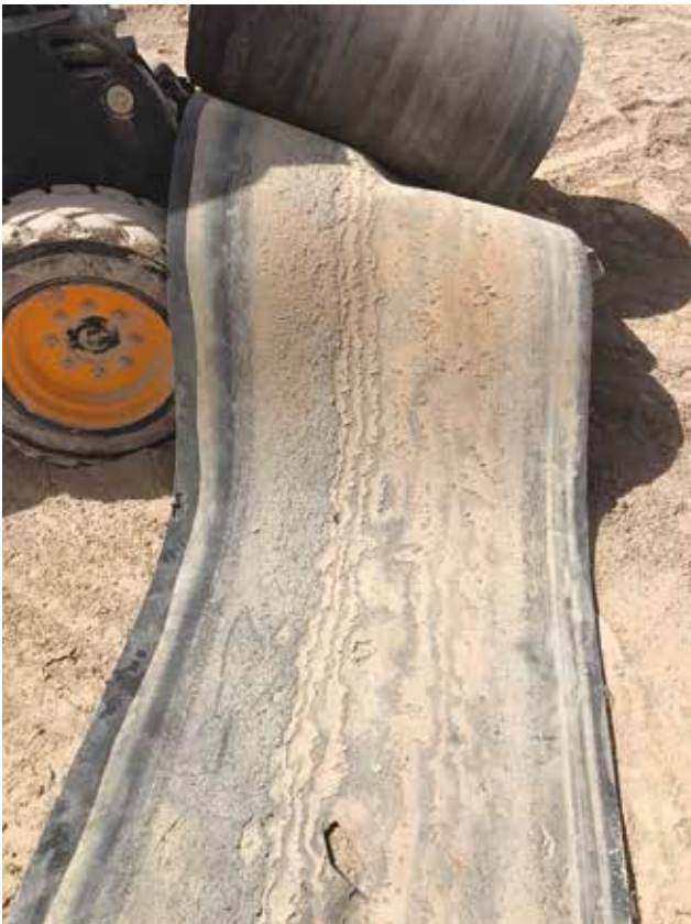
On the scrap heap after only 600 hours. There can be a very big difference between one conveyor belt and another.
