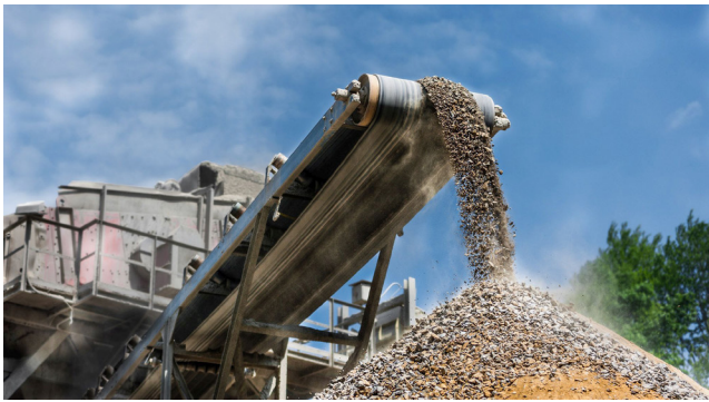
Figure 1. Abrasive material is effectively 'accelerated' across the belt surface.
