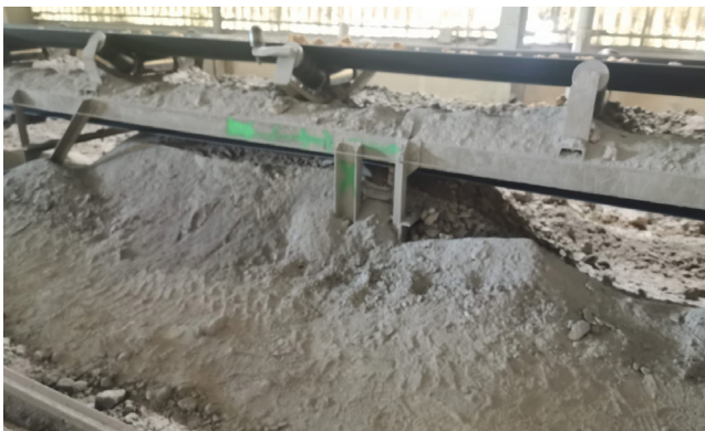
Figure 3. Pollution problems – fine particles of dust penetrate the cracks and are then shaken out on the return run of the belt.
