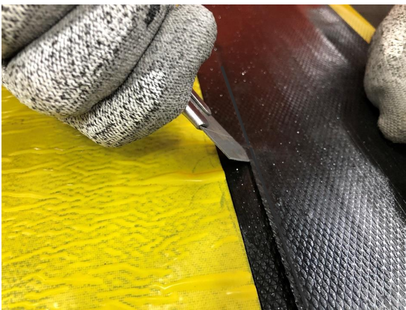
Photo 20: Cutting of bottom cover to size
