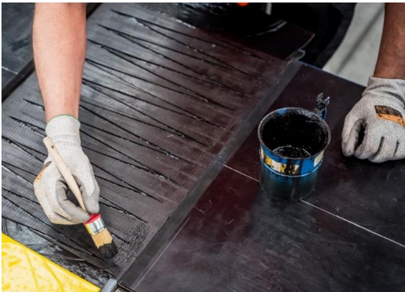
Photo 23: Solution on top of fingers
