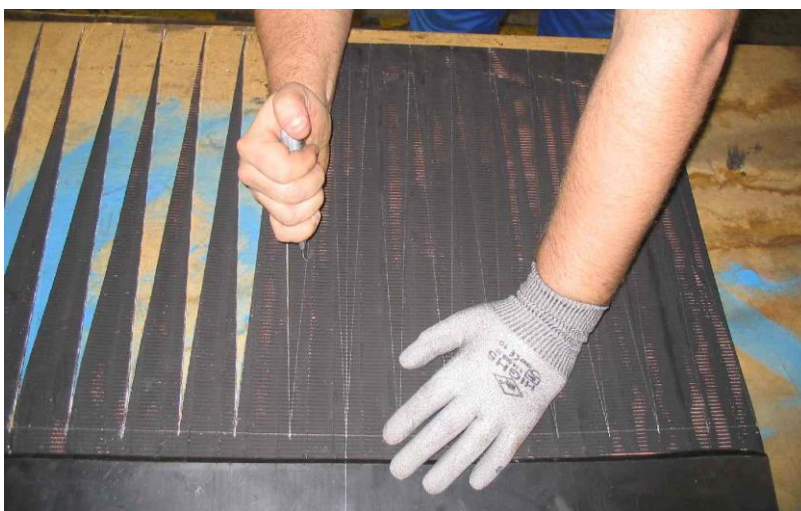
Photo 9: Cutting the fingers
