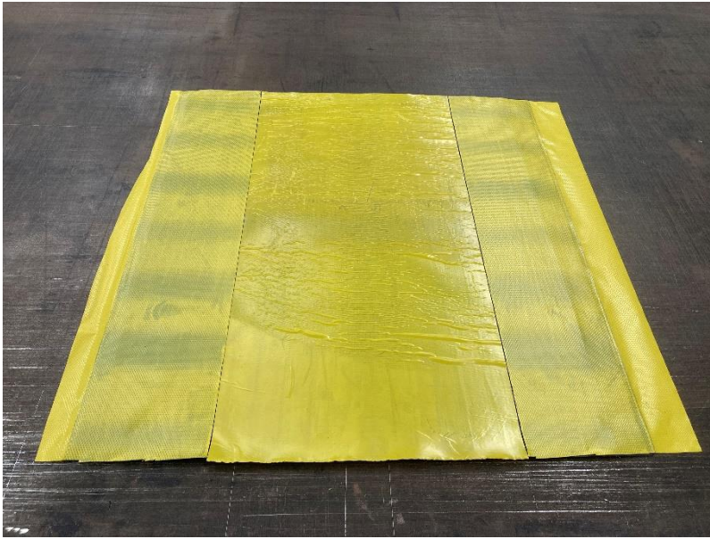
Photo 17: Applying two skim layers next to the fabric
