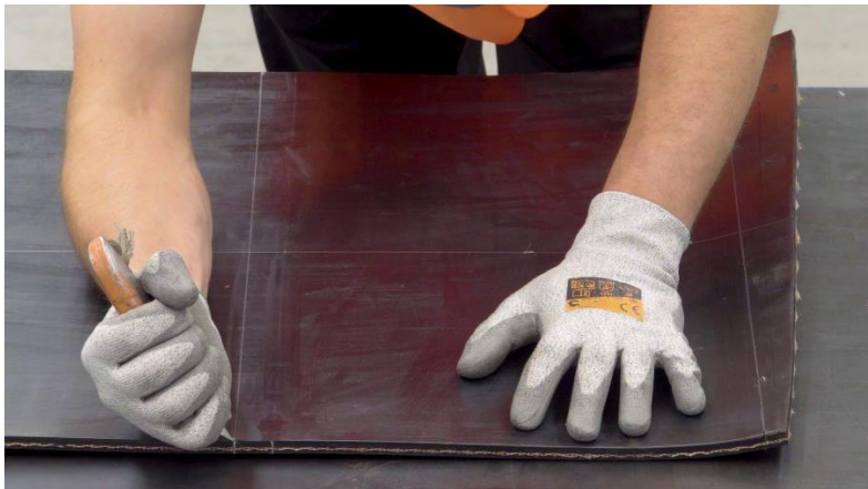
Photo 2: Cutting at an angle of at least 45°
