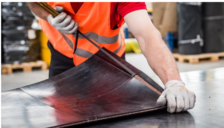
Photo 3: Cutting and removal of the cover
