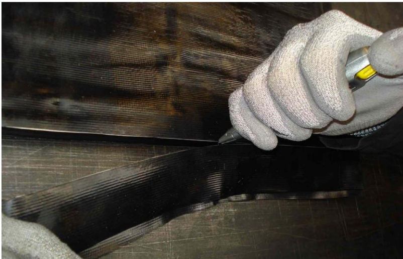
Photo 28: Trimming of the edges
