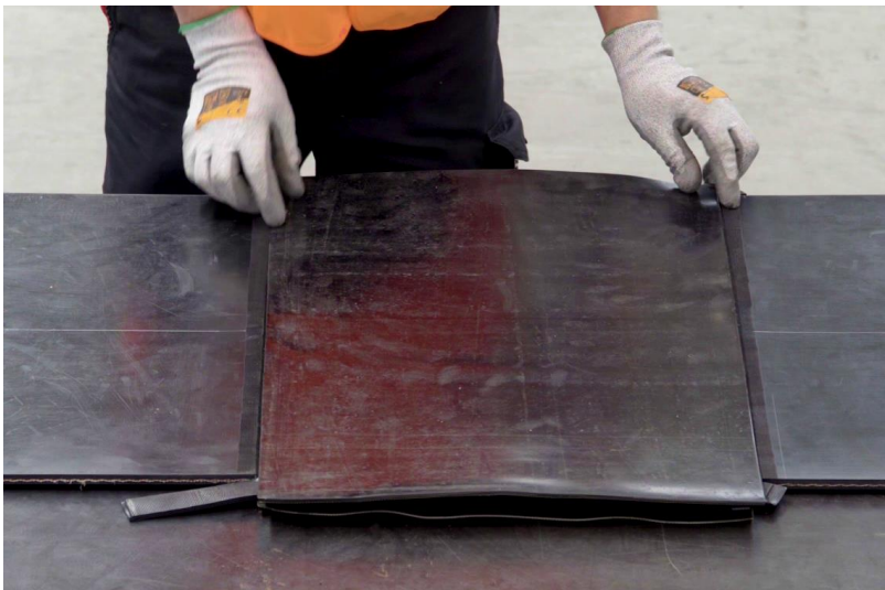
Photo 30: Applying the top cover
