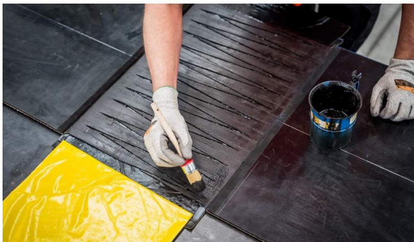
Photo 21: Solution on top of fingers
