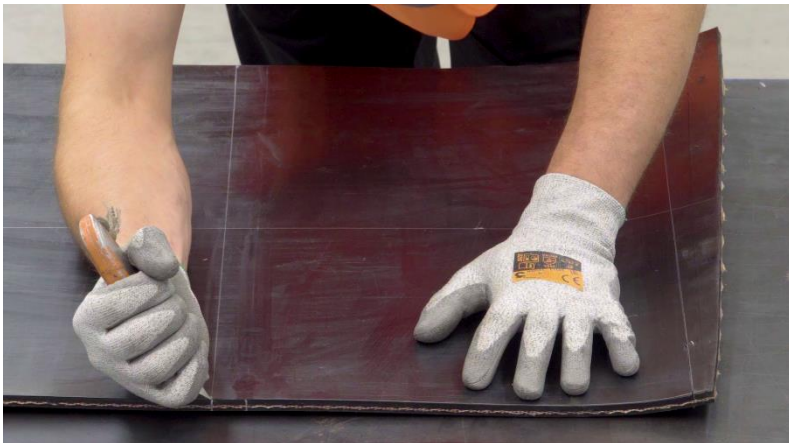
Photo 2: Cutting at an angle of at least 45°
