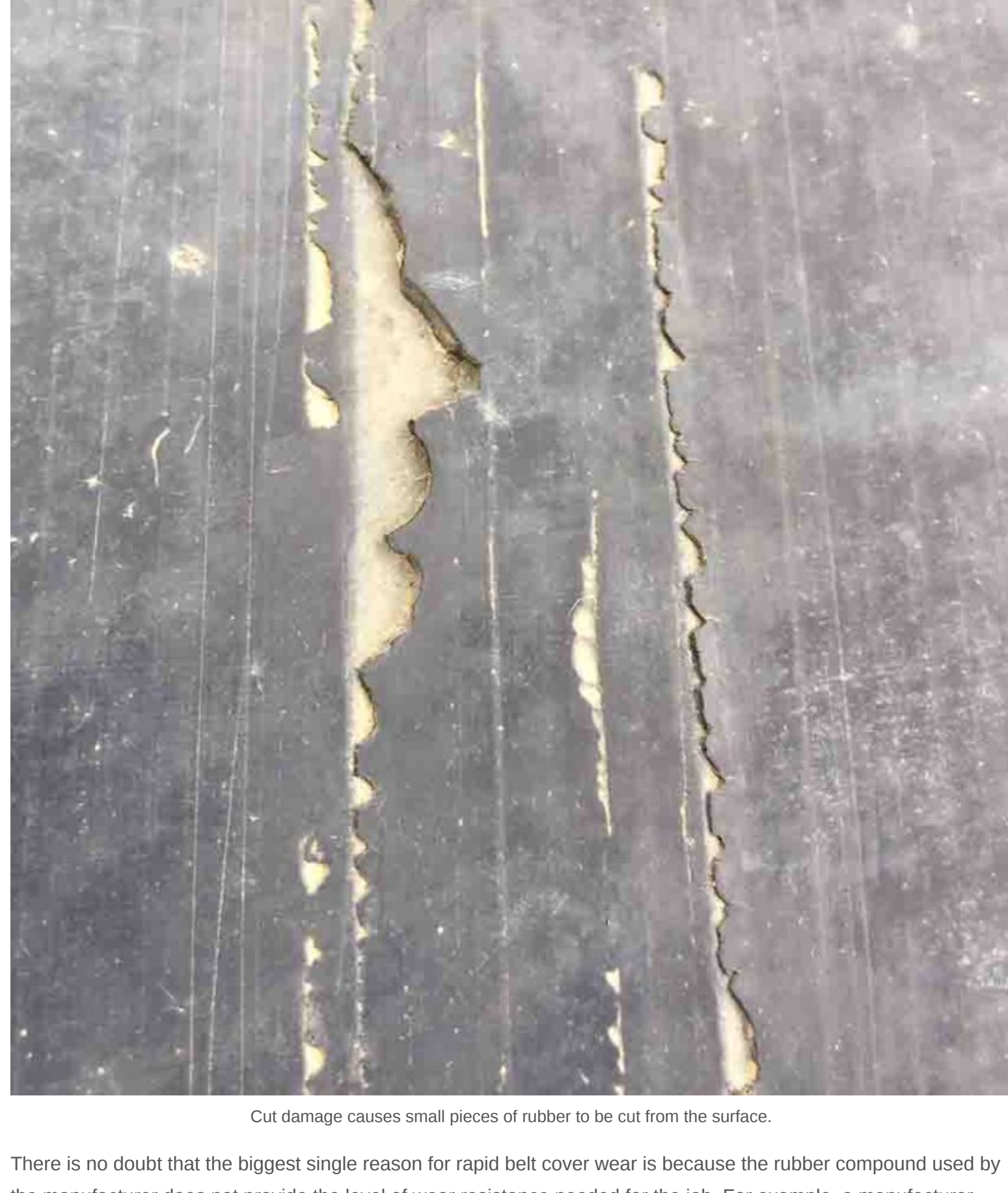
Cut damage causes small pieces of rubber to be cut from the surface.
