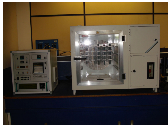
Ozone testing cabinet. Image courtesy of Fenner Dunlop, The Netherlands.
