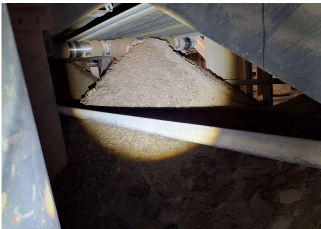
Figure 2. Waste build-up is a common sight and causes a lot of avoidable wear and stoppages.
